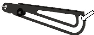
Figure 11: Indication of the final clamping bracket guide in which the bushing must slide to prevent accidental door closing.
